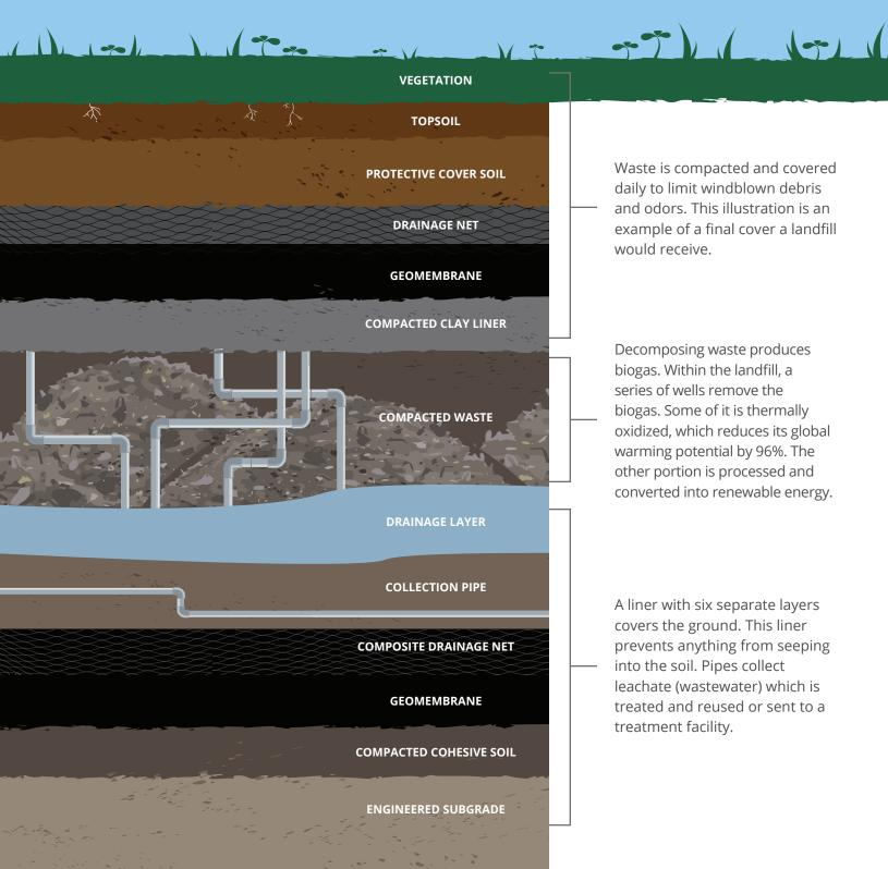
Waste is compacted and covered daily to limit windblown debris and odors. This illustration is an example of a final cover a landfill would receive.
